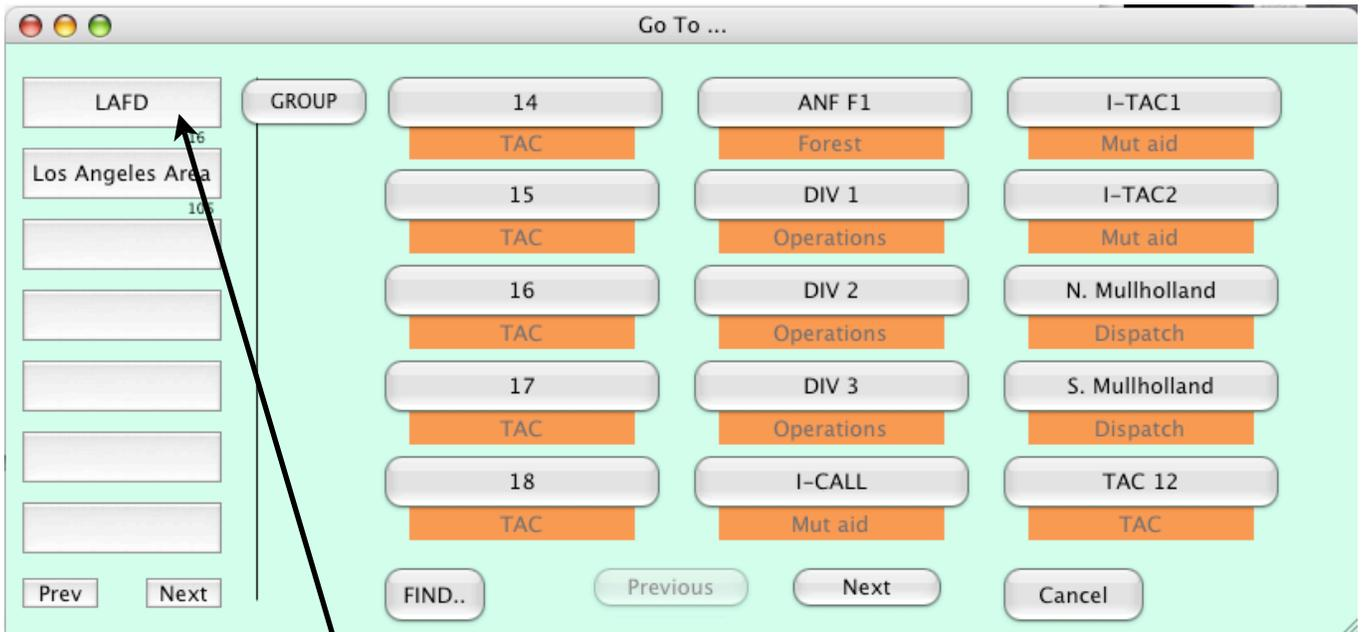
Pressing the SYSTEM button (LAFD) creates a channel list of all the LAFD channels in order of Channel name. The names in the orange tags are groups that were programmed into that SYSTEM.
